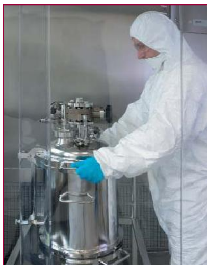
Laminar flow cabin and hastelloy pressure filter (above) and newly built cGMP kilo lab (below) at Solvias's site in Basel
